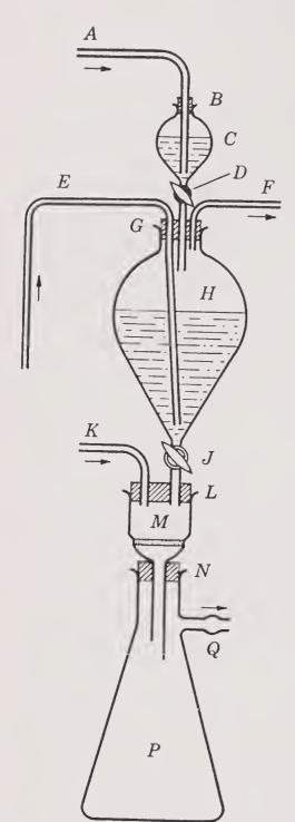
Fig. 1. Apparatus for preparation of alloxantin dihydrate.
